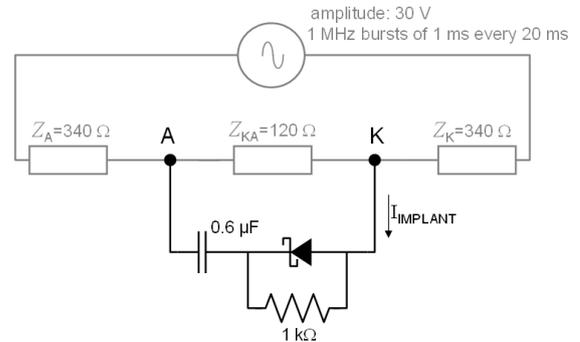
Figure 2: Proposed circuitry to perform charge balance (in black). The indicated numerical values have been chosen for reproducing the experiment performed with the implemented prototype (section III).
