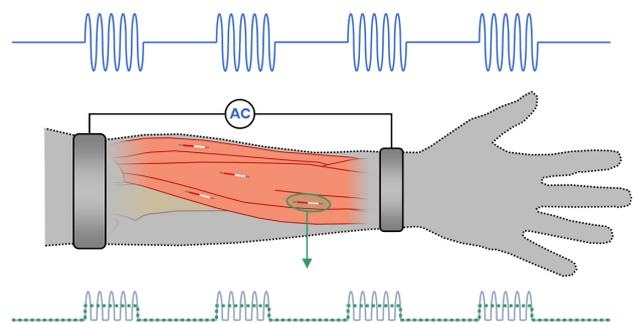
Figure 1: The proposed technology is based on externally applying an inert HF current which is rectified by the implants into LF currents capable of stimulation.
