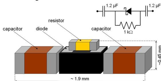
Figure 6: Electronic component placing (and the circuit formed after soldering). Two capacitors are employed in order to double the voltage tolerance ( $6.3 \text{ V} + 6.3 \text{ V}$ ) and for geometrical symmetry.
