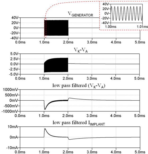
Figure 3: SPICE simulation results for the circuit in Fig. 2.
