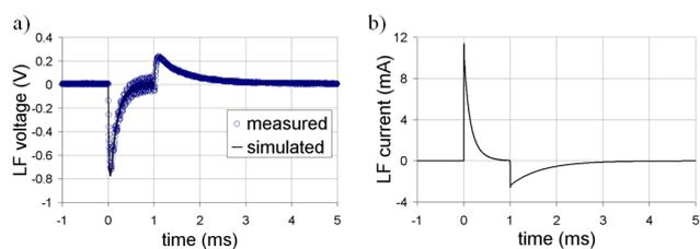
Figure 7: (a) Voltage recorded across the prototype's electrodes and its comparison to simulated voltage. (b) Simulated current for this scenario.
