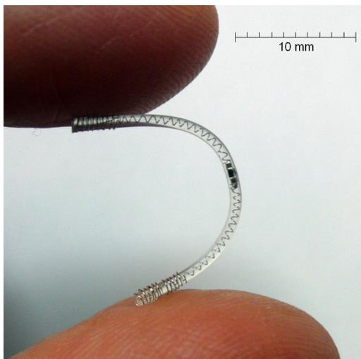
Figure 5: Implemented prototype. The electronic components and the two connections to the electrodes are contained within a silicone body. Both the connections and the electrodes consist of coiled Pt-Ir wires.
