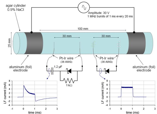
Figure 4: Setup for charge balance demonstration. The proposed circuit is compared to a circuit consisting of just a diode. (References for the components are noted in section III.A)
