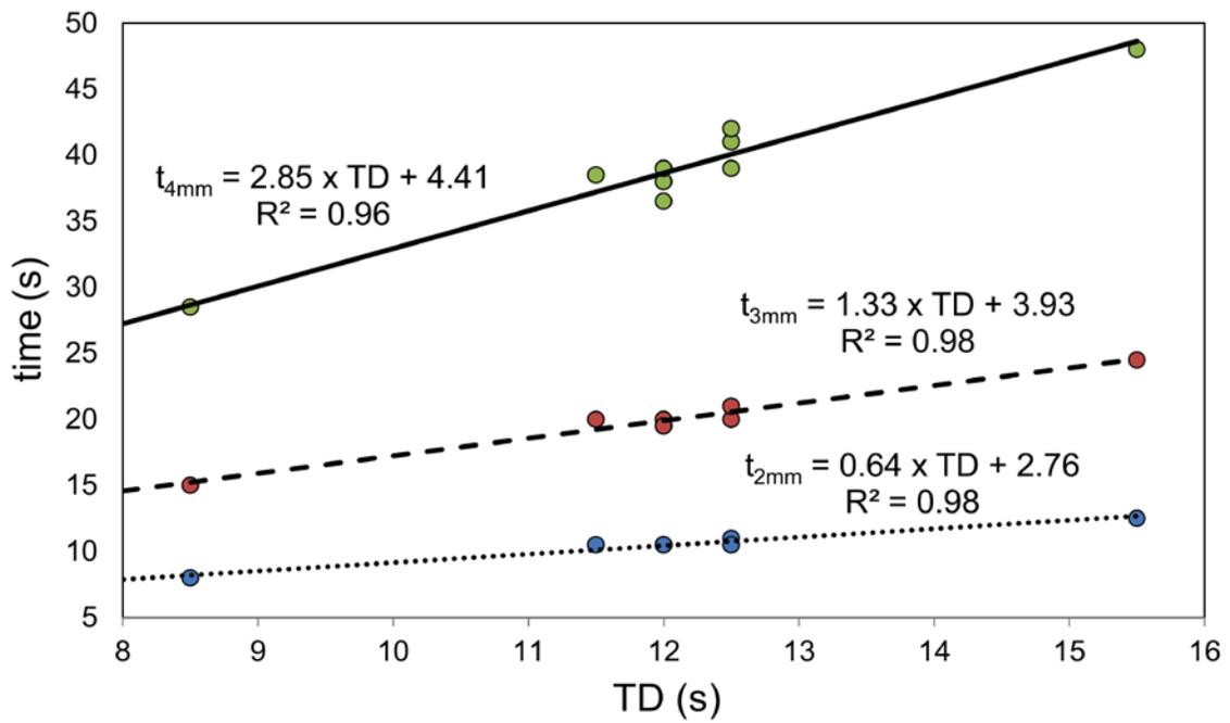
**Figure 7** Relationship between the time when ISO-70°C reaches a depth of 0.75 mm (TD) and the time required to achieve a lesion depth of 2 mm, 3 mm and 4 mm ( $t_{2\text{mm}}$ ,  $t_{3\text{mm}}$  and  $t_{4\text{mm}}$ ).
