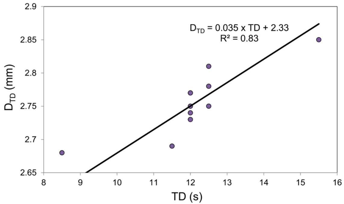
**Figure 6** Relationship between the time at which the 70°C isotherm reaches a depth of 0.75 mm (TD, denaturation time) and thermal lesion depth at that time (D<sub>TD</sub>).
