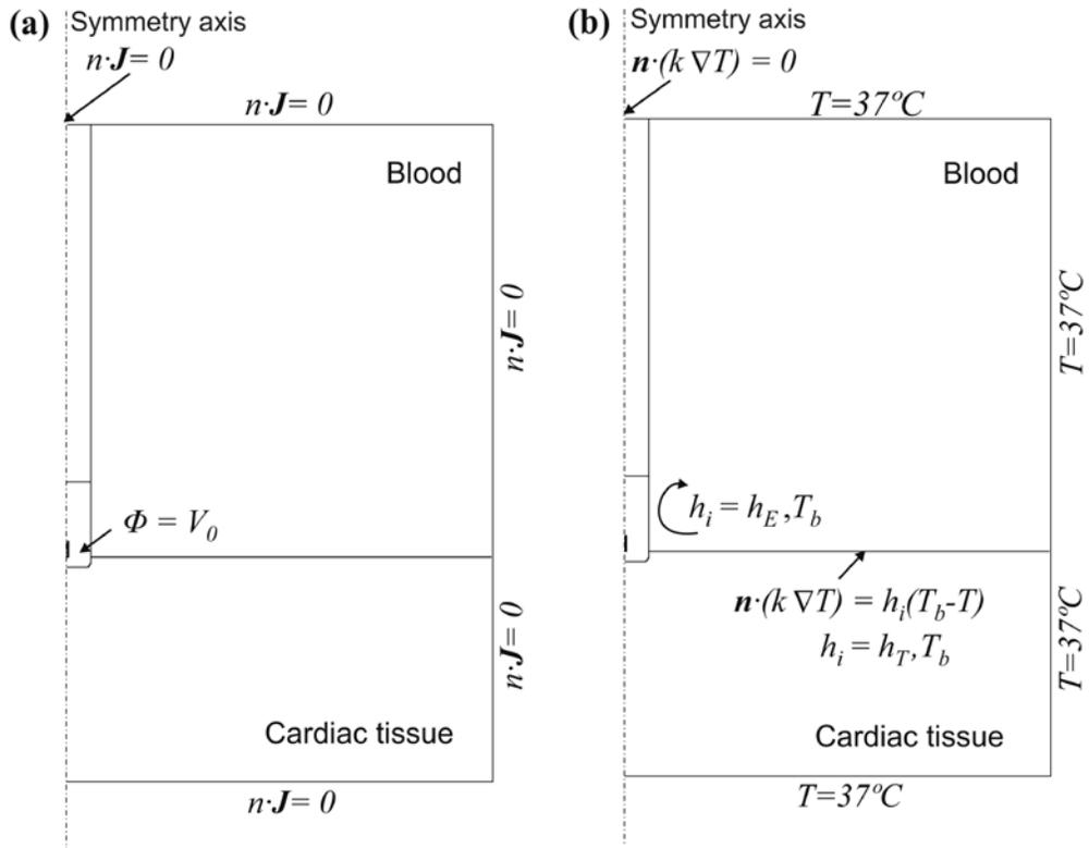
**Figure 2** Electrical (a) and thermal (b) boundary conditions of the model.  $h_E$  and  $h_T$  are the thermal convection coefficients at the electrode–blood and the tissue–blood interfaces, respectively.
