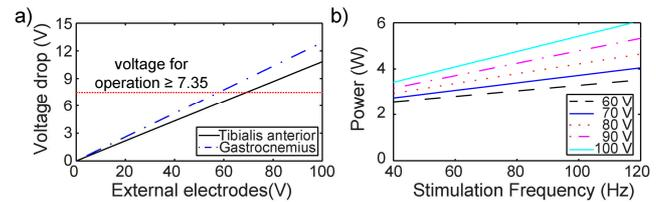
Fig. 3. Parametric simulation results. a) Voltage amplitude across implant electrodes. b) Power consumption of the external system when the implants are used for continuous stimulation, modeling different input voltages and stimulation frequencies (i.e. bursts frequency).
