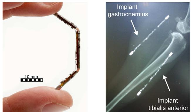
Fig. 1. Addressable neuromuscular stimulator reported in [1]. The X-ray image shows two implants in a rabbit leg. Much thinner and more flexible versions are conceivable by embedding all circuitry in a single integrated circuit.
