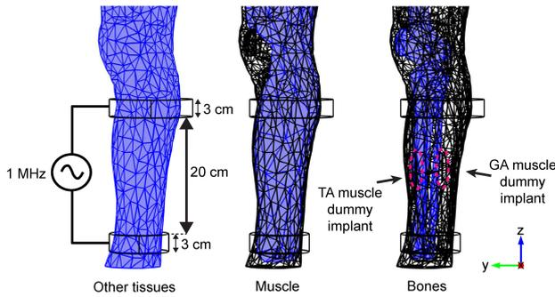
Fig. 2. Leg model, corresponding to a male adult, used in the simulations. Two external electrodes are modeled around the limb, and two dummy implants are modeled in the tibialis anterior (TA) and gastrocnemius (GA) muscles.
